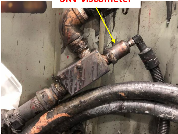
Showing the inline installation of the Rheonics SRV viscometer in an ink delivery system
