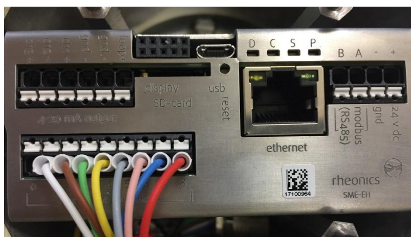
Figure 8: Sensor cable connection to the sensor electronics.
