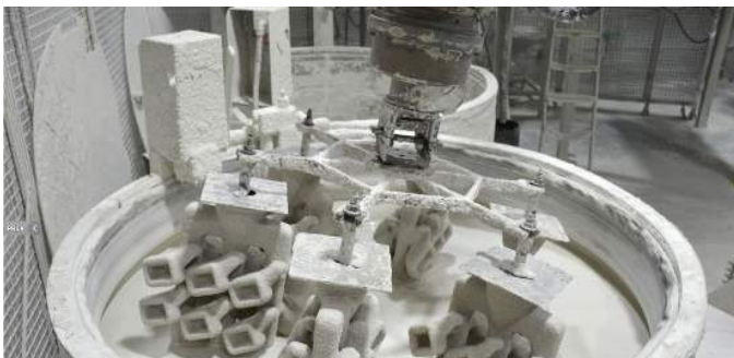
Continuous Drum Slurry Monitoring
