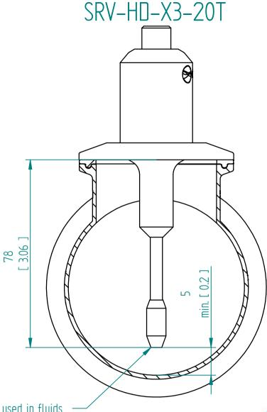
This accessory should not be used in fluids and applications where there is a chance of plugging at the base of the sensor.
