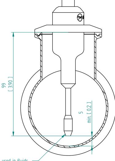
This accessory should not be used in fluids and applications where there is a chance of plugging at the base of the sensor.
