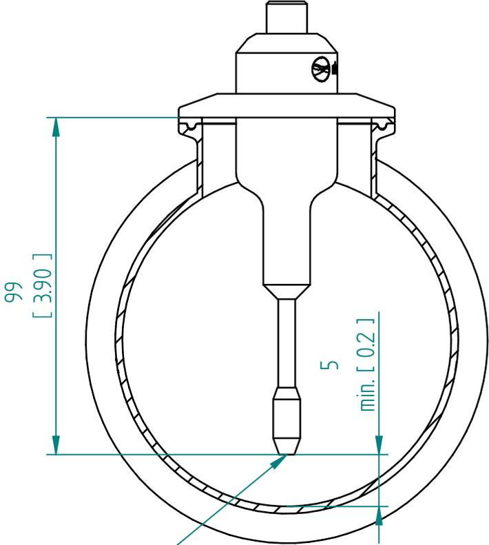
This accessory should not be used in fluids and applications where there is a chance of plugging at the base of the sensor.
