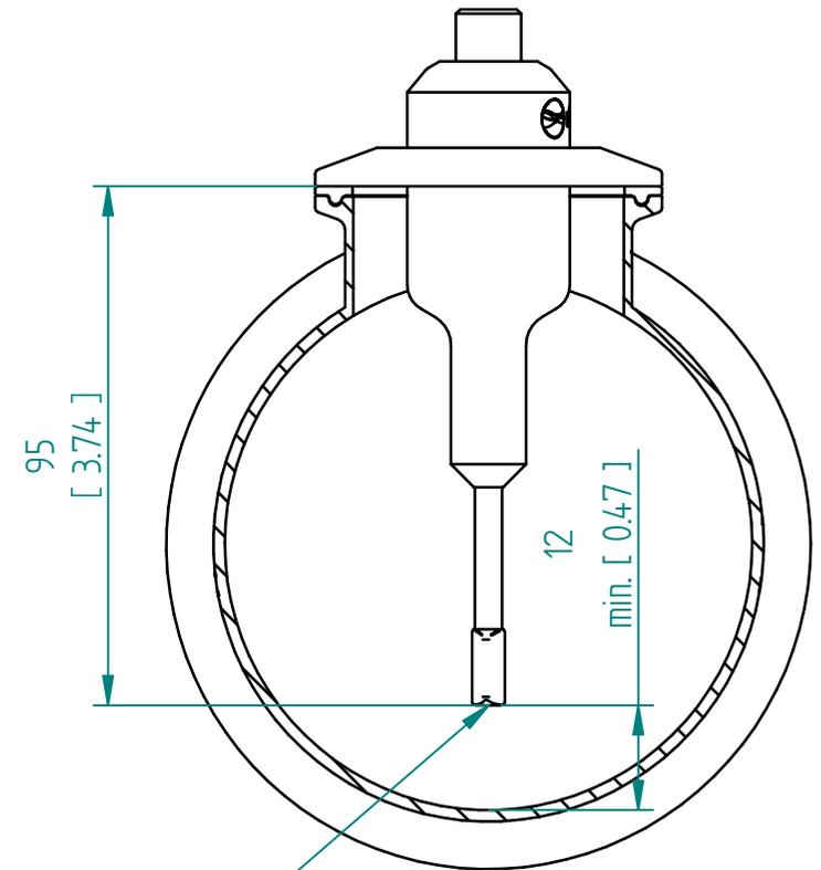
This accessory should not be used in fluids and applications where there is a chance of plugging at the base of the sensor.
