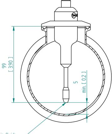
This accessory should not be used in fluids and applications where there is a chance of plugging at the base of the sensor.
