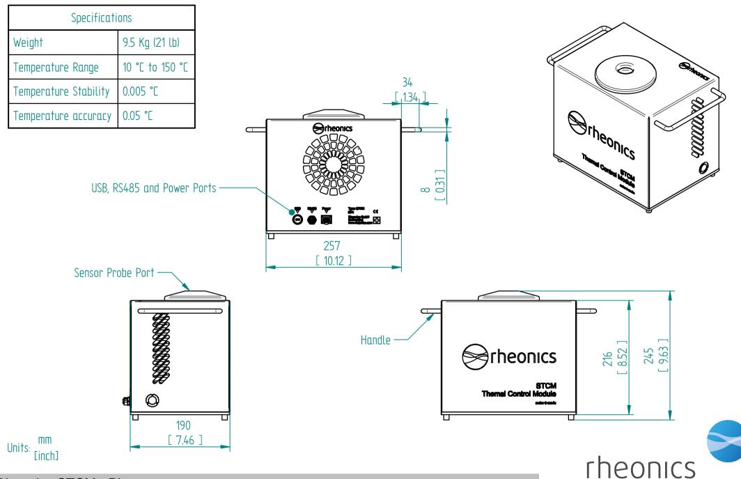
Rheonics STCM - PL Type-SR Thermal Control Module
