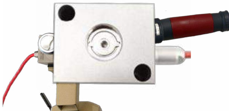
Figure 18: Using a wrench to remove DV sensor from DVM
