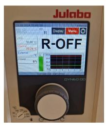
11. Move the lever to the left. This will set the bath to "external circulation" as is needed to operate the DCM-BB.
