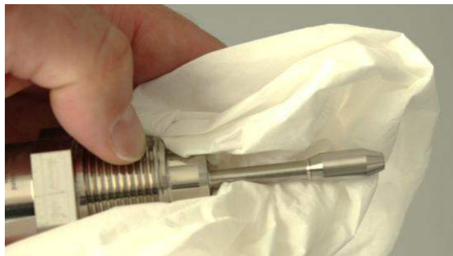
Figure 13: Cleaning the sensor with solvent-saturated cloth or paper.
