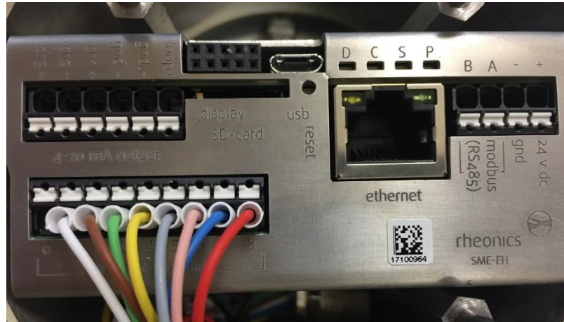
Figure 8: Sensor cable connection to the sensor electronics.
