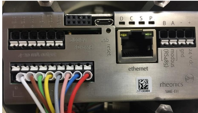
Figure 8: Sensor cable connection to the sensor electronics.
