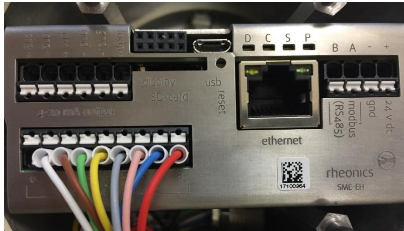
Figure 12: Sensor cable connection to the sensor electronics.
