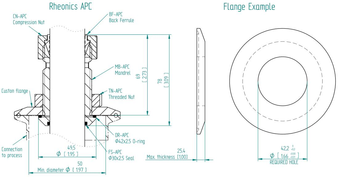
Units: mm [inch] For compatibility with APC, the flange should comply with max. thickness, and inner hole with defined dimension.
