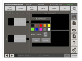
The 'Auto' button has two functions: selects current measured viscosity value as the setpoint and enables automatic control across the coating run.
