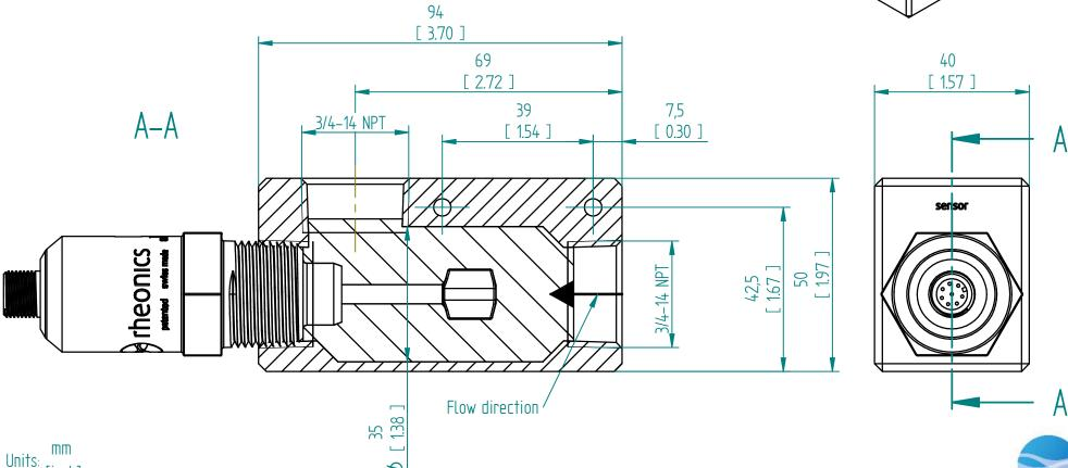
SRD 3/4" NPT Inline Flow Cell IFC-34N-SRD
