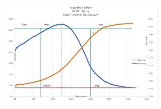
Fig. 3: CureTrack curing curves of a fast-curing consumer epoxy adhesive Pacer Pt39 Z-Poxy. Plot shows the damping and frequency of the CureTrack with Liquid, Gelled and Solid-Cured phases of the adhesive.
