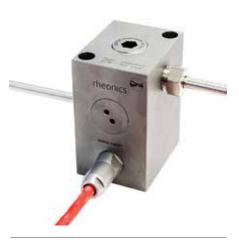
The Rheonics DVM is well-suited to measuring properties of live oil samples, because of its small sample volume, its wide range of viscosity measurement without interrupting a measurement run to re-configure the hardware, and its ability to measure density and viscosity simultaneously on the same sample, Fig. 6. Because competing systems use two separate instruments to measure density
